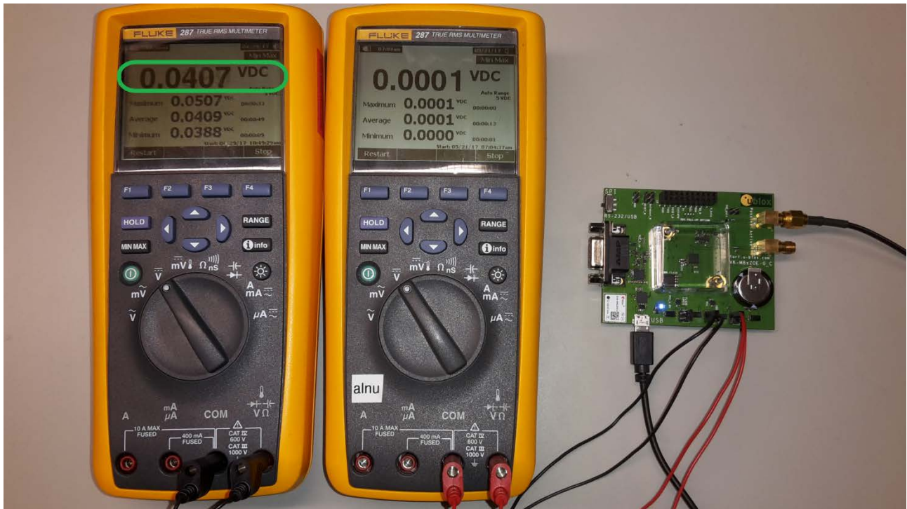
Figure 9: Setup to measure the VCC current consumption of ZOE-M8B on EVK-M8BZOE
