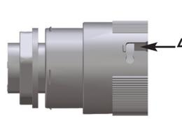
3702/V...: socket (3) with holes for fixing (4) and gland
