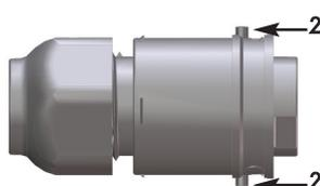
3702/A...: plug body (3) with openings for clamping (4)
